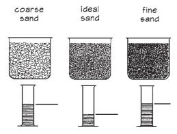
The level of liquid in the cylinders represents the volume of voids in the sand mixture. A sand with the ideal mix of coarse and fine grains (complying with ASTM C144 gradation limits) has a lower volume of voids and is therefore more economical because it requires less cementitious material to properly coat the particles.
